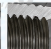
Thread machining (API 7-2 / ISO 10424-2)
