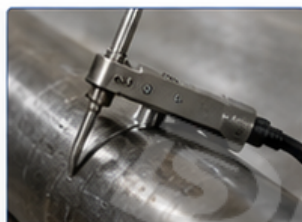
Wall Thickness Measurement
